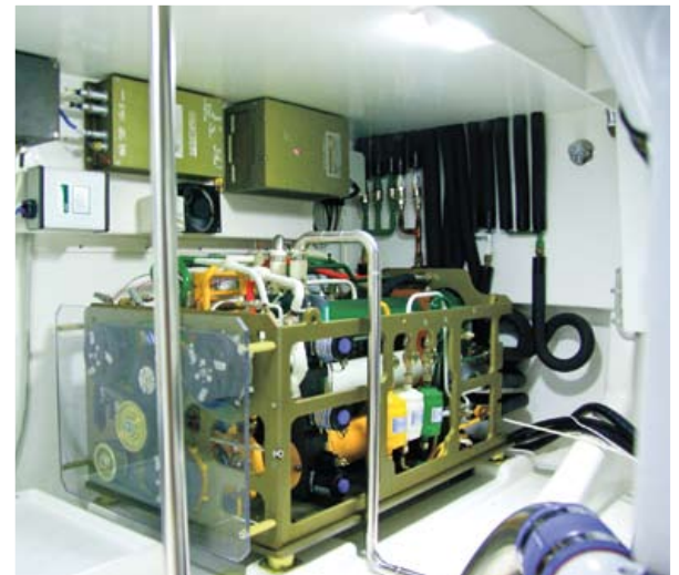
Above: This JEC Combi VI unit sits snugly in the engine room of the O'Brien 56 Sportfisherman Kekōa (shown at top).
